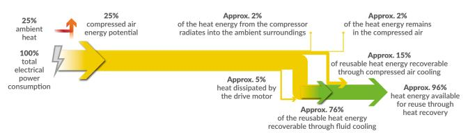
The fully-enclosed design of modern rotary screw compressors makes them well suited to the heat recovery process. Both fluid-injected and oil-free compressors can be used. Advantages of our heat recovering technology include:
