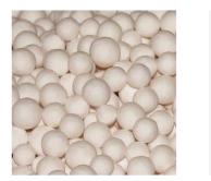
High quality molecular sieve ensure long service interval. Molecular sieve is also protected from unexpected liquid intake.
