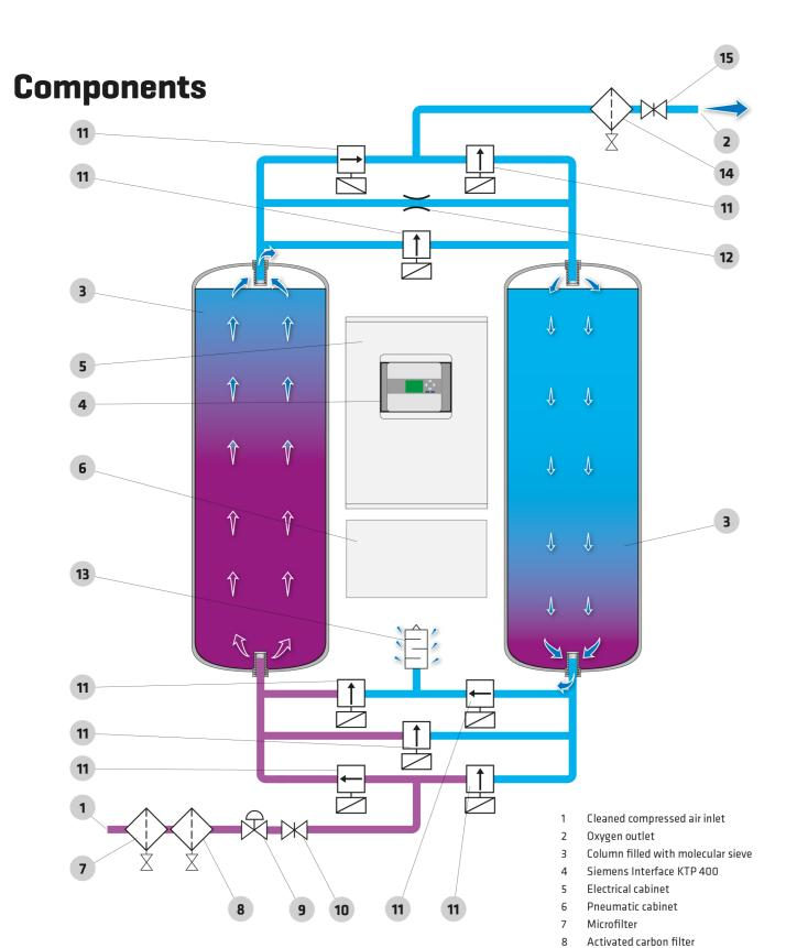
The O-GEN series oxygen generators extract production cycle. In order to guarantee a constant pass through as a product gas, but adsorbs other have an almost indefinite lifetime. gases. The sieve releases the adsorbed gases to the atmosphere, when the outlet valve is closed and the bed pressure returns to ambient pressure.
